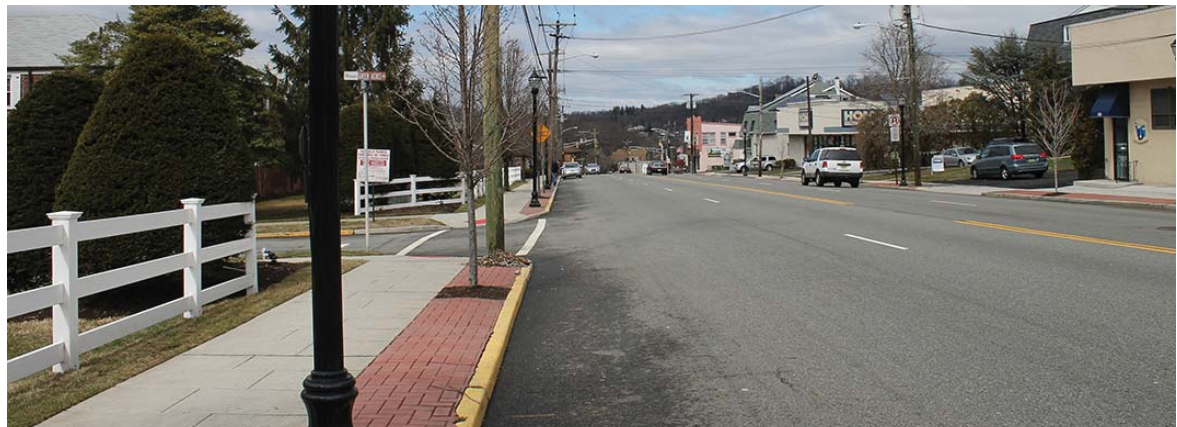
Bloomfield Avenue, particularly in areas outside the downtown cores like this section in Verona, experience speeds much higher than the posted limits often due to the perception of such a wide roadway.
