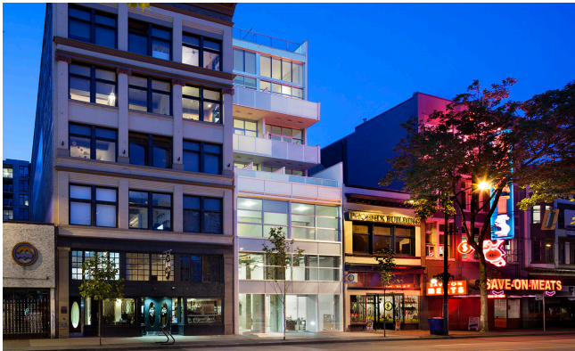
A.5-01: Encouraged: Carefully designed stepbacks in midrise buildings can produce matching rooflines between historic structures and larger, stylistically different neighbors. Buildings utilizing stepbacks are perceived as smaller by pedestrians.
