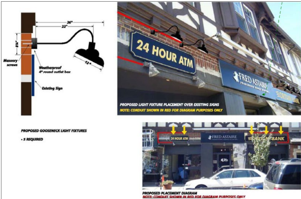
Figure 3: Sample of Lighting Details
